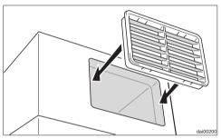
Only for recirculation: With the slats pointing downwards, install the recirculation vents through the extension piece and into the diverter.
